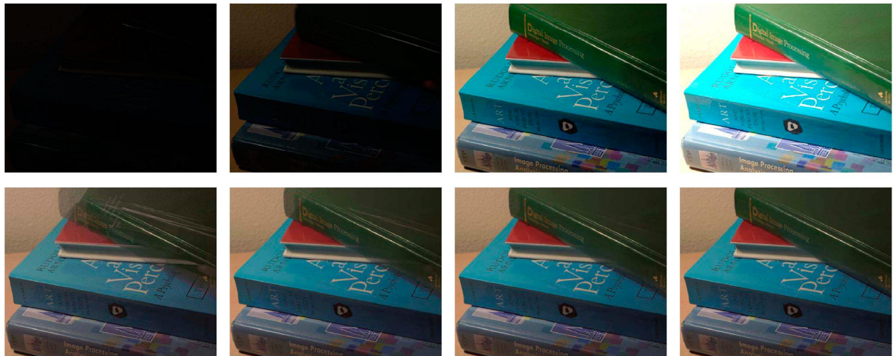
Fig. 4. The top row shows the second, fourth, sixth and eighth exposures of a sequence in which a book is being placed upon a stack of books. The bottom row (left to right) shows tonemapped HDR images that were generated using weights determined only by absolute pixel values, and weights that were estimated with one, two, and fourteen iterations of our algorithm.
