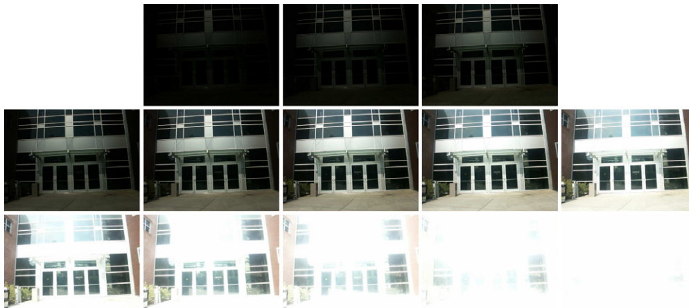
Fig. 10. Image sequence used to create the response curve of the Minolta camera. The same scene is captured also with the Nikon camera to recover its response. The sequence is captured by using a tripod to minimize alignment problems. The exposure times from darkest to lightest exposure vary from \frac{1}{16,000} to \frac{1}{4} s, with doubling at each exposure.
