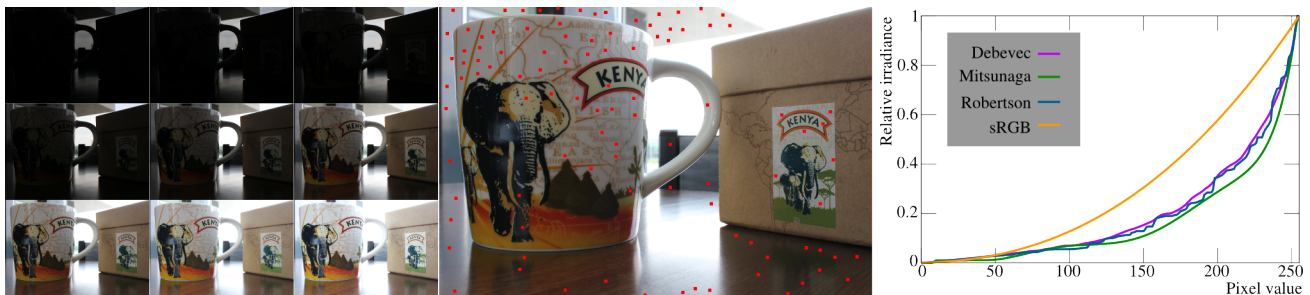
Figure 1: The response of a Canon EOS 550D is recovered with three methods (right) using the samples (middle) from the exposures (left).
