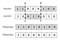
Figure 4. Crossover operator that produces two offsprings from two selected individuals
