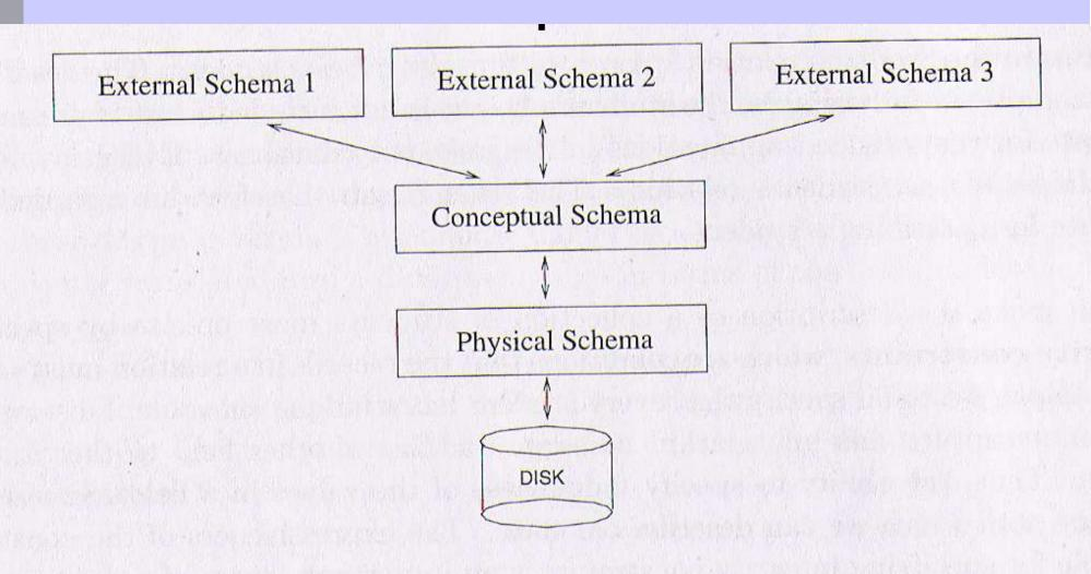
Figure 1.2 Levels of Abstraction in a DBMS
