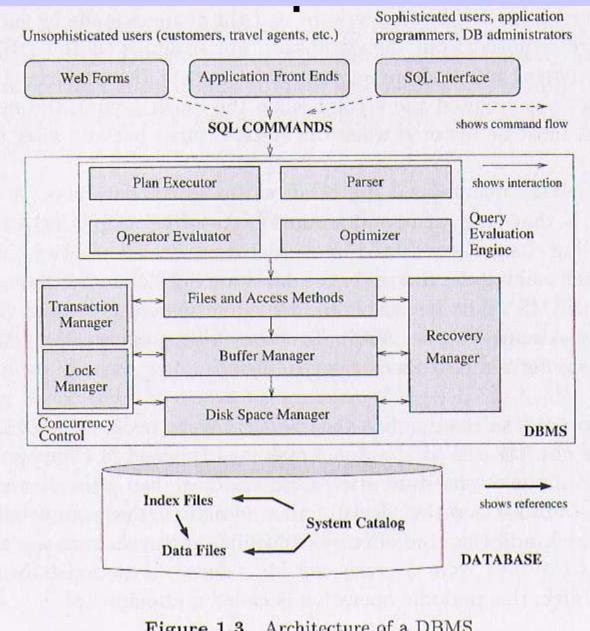
Figure 1.3 Architecture of a DBMS
