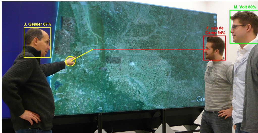
Figure 6. Example: interaction with our videowall through hand gestures and head pose
