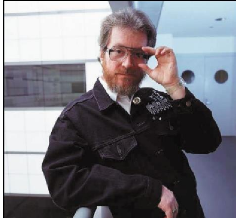
Figure 4. The author wearing a variety of new devices. The glasses (built by Microoptical, Boston) contain a computer display nearly invisible to others. The jacket has a keyboard literally embroidered into the cloth. The lapel has a context sensor that classifies the user's surroundings. And, of course, there's a computer (not visible in this photograph).
