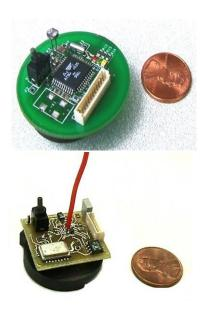
RF 916.5 MHz OOK 10kbps 20 meter range Sensors: light, temperature
