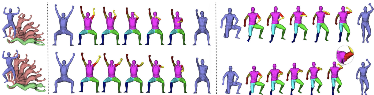
Fig. 12. Spherical linear interpolation (SLERP) of quaternions (left bottom) produces a rotation with more uniform velocity than LERP does (left top) and hence is preferred for this test. Note that, SLERP to the quaternions are applied over a Bezier curve, not separately. (Middle and right) Quaternion interpolation, however, is prone to errors at joints (bottom rows) when acting on multiple parts, a problem we avoid by our original algorithm (top rows). Average V and P values over 20 SCAPE runs are 53 and 0.8, respectively, which are worse than the corresponding entries of our original algorithm (Table 2).
