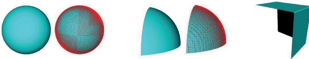
Figure 13. Ground-truth sphere surface obtained by subdividing an initial tetrahedron (left pair) that has the same smoothness as our resulting sphere isosurface extracted from the FCC lattice (middle pair). Another smooth surface from our method matches the ground-truth planes (rightmost).
