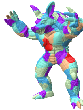
Fig. 5. The partitions running at the same time are marked with the same color, where each color represents a different thread batch.
